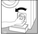
Unscrew and remove the filter.
